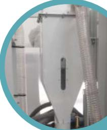
The cyclone can download the aspirated material in a tank or directly in the IBIX® blasting machine. The cyclone may be equipped with riser rails with pneumatic cylinder, or fixed in the upper position (see layout). Thus, the dust container (05) can be positioned beneath the cyclone or the IBIX® blasting (06) machine.
